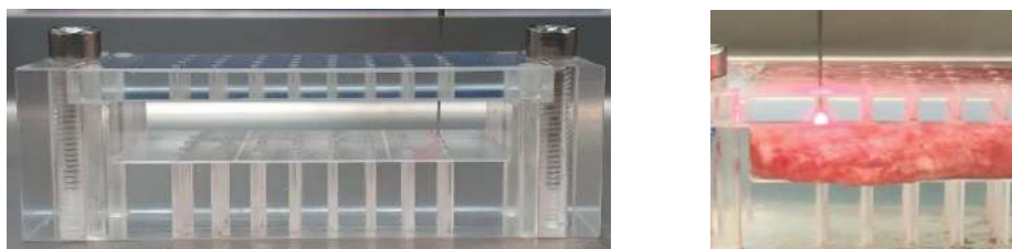
Supplementary Figure.4 | Experimental setup for determination of the depth resolution of the fiber-optic needle
