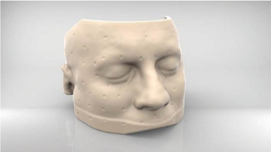
**Figure 2. The final phantom head design, with 90 surface divots.**
