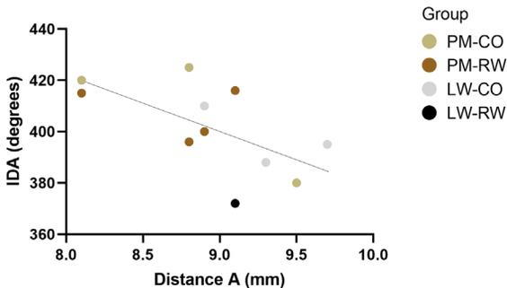
**Figure 11.** The insertion depth angles and corresponding cochlear distance A are plotted of the 11 full insertions according to the manufactures guidelines. An inverse correlation is observed between insertion depth angle and distance A ( $R^2 = 0.39$ ,  $p < 0.05$ ). Distance A is an indirect measure of cochlear duct length. IDA: insertion depth angle; PM: perimodiolar; LW:lateral wall; CO: cochleostomy; RW: round window.
