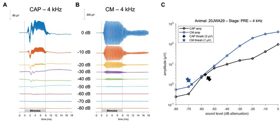
**Figure 4.** Example of a compound action potential (CAP; A) and a cochlear microphonics (CM; B) response to a 4 kHz tone across different sound levels. Stimulus started with maximum sound level (in this instance of 4 kHz, at 104 dB SPL) and was attenuated in 10 dB steps until the CAP or CM response was not visible anymore. Subsequently, an input/output curve was constructed, and the threshold was interpolated using pre-defined threshold criteria (C).
