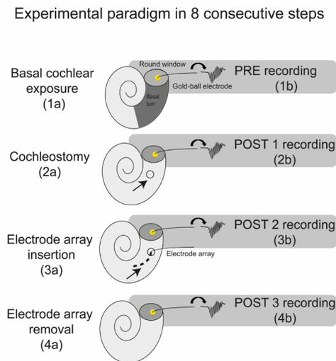
**Figure 1.** A schematic overview of the experimental paradigm. The electrocochleography was performed using the gold-ball electrode in the round window niche. The experiments consisted of 8 consecutive steps, with electrocochleography at 4 separate stages of the procedure, i.e. at PRE (before cochleostomy), POST1 (after cochleostomy), POST2 (after electrode-array insertion) and POST3 (after electrode-array removal).
