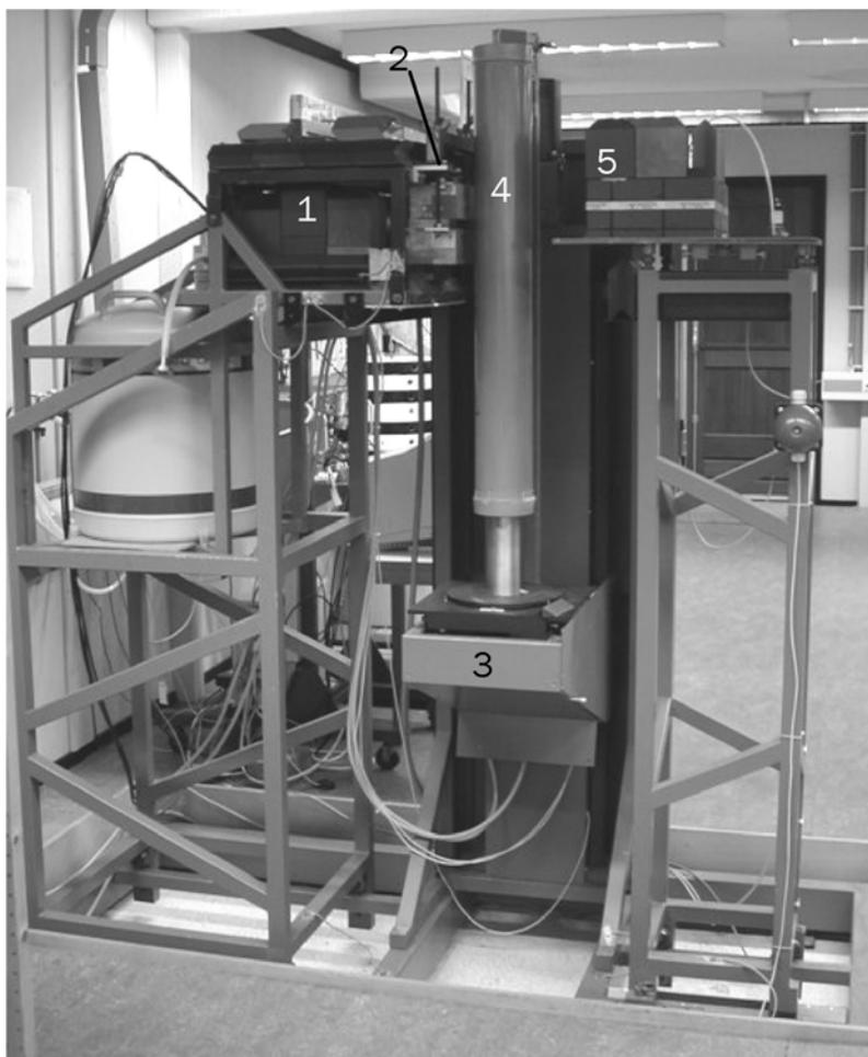
*Figure 4 The measurement set-up during a scan of a 1 m high sample. indicated are (1) the detector in a lead shielding, (2) the collimator, (3) the sample holder, (4) the sample and (5) the lead castle that contains the transmission source. A schematic drawing of detector, collimator, stepper motor movement options and sample is given in the next figure.*
