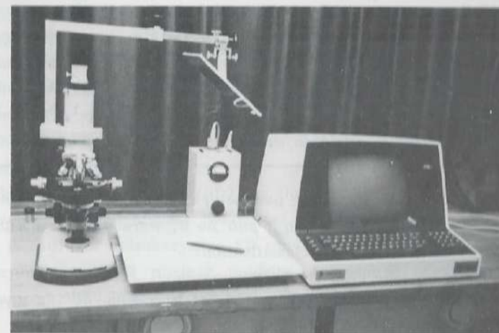
Fig. 2 Technical equipment: At the centre the digitising tablet on which the microscope image is projected by a mirror. On the right the standard computer terminal on which the results are shown. The average time to measure 50 cells is 15 min.
