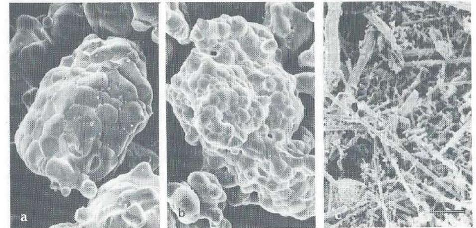
Fig. 1 a - c. Scanning electron micrographs of the three materials under study. a: hydroxyapatite, b: tri-calcium phosphate, c: crocidolite asbestos. Bar: 5  $\mu\text{m}$ .
