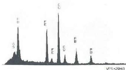
Fig. 4. X-ray microanalysis spectrum of one of the inclusion bodies in 3b (arrow), showing the presence of iron. (Vertical full scale 2,048 counts.)
