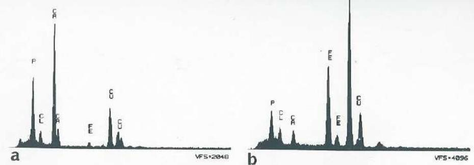
Fig. 9, a and b. X-ray microanalytical spectra of the deposit in Fig. 8c.
