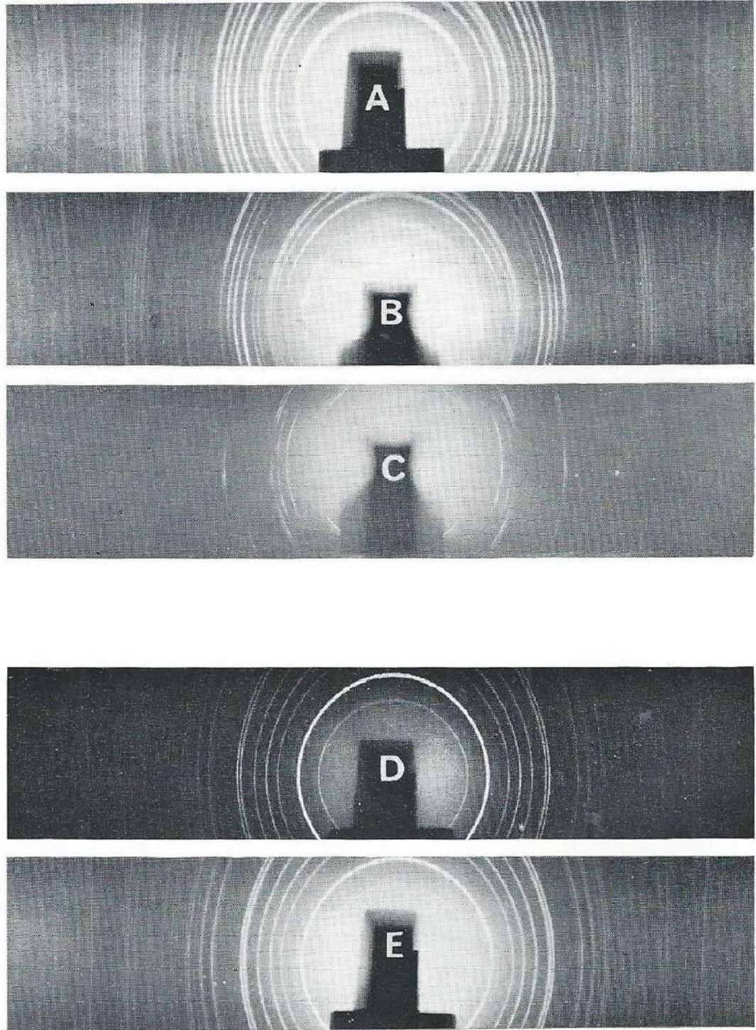
X-ray diffraction patterns. **A**, aragonite standard; **B**, fragment of the statolith of the pike; **C**, small splinter of the statolith of the pike; **D**, calcite standard; **E**, statoconia of the mouse.
