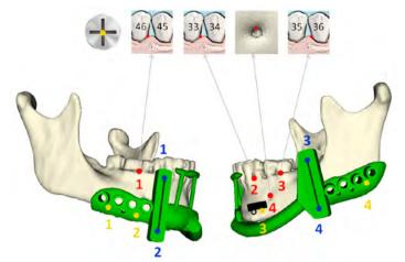
**Figure 3** Schematic model of a mandible with the cutting guide (green). The sensor housing module (black) is fixated on the part of the mandible that will be resected. The yellow landmarks are used for fiducial registration. The anatomical landmarks (red) are located on teeth and mental foramen. The landmarks at the cutting guide (blue) are located in the upper and lower ends of the sawing slots. Dental numbering according to the FDI World Dental Federation (ISO 3950).
