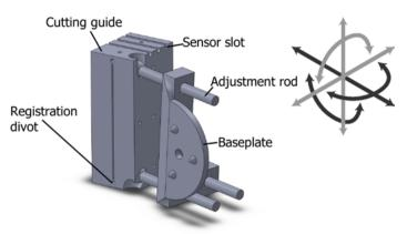
Figure 1 3D model of the navigated cutting guide, dubbed "Bladerunner". In the upper right corner, displayed in black are the 3 degrees of freedom.
