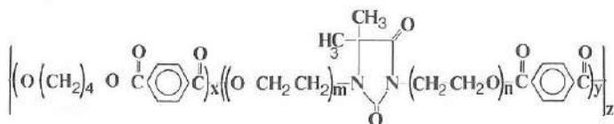
Fig. 4. Chemical formula of HPOE/PBT segmented copolymer.
