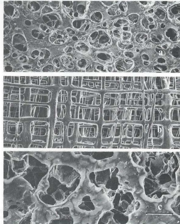
Fig. 1. Scanning electron micrograph of the surface of three biomaterials: (a) Estane<sup>R</sup>, (b) polypropylene oxide, and (c) the HPOE/PBT copolymer. Note the relatively rough surface of Estane compared with that of polypropylene oxide and copolymer. Bar = 100  $\mu\text{m}$ .
