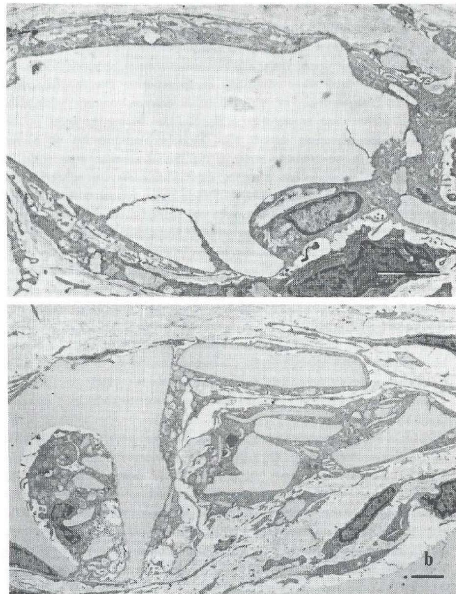
Fig. 9. Transmission electron micrographs of tympanic membrane implants showing HPOE/PBT copolymer fragmentation; (a) 13 and (b) 26 weeks post-operatively. Bars = 6  $\mu$ m.
