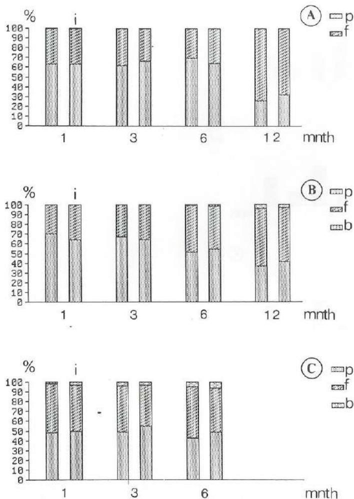
Fig. 5 (a-c). Course of the percentages of implant-surrounding tissue occupied by phagocytes (P), fibrous tissue (F), and bone (B) without infection (right bars) and with infection (left bars; i). Values are means of the total number of samples of Estane<sup>R</sup> (a), polypropylene oxide (b), and copolymer (c).
