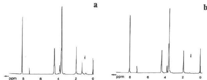
Fig. 5a and b. NMR-spectra of 55/45 HPOE/PBT copolymer. a: Spectrum of un-purified copolymer. Note the two peaks between 0.8 and 1.3 ppm (arrows) suggestive of low molecular weight impurities. b: Spectrum after purification. Peaks as in a (arrows) are absent.
