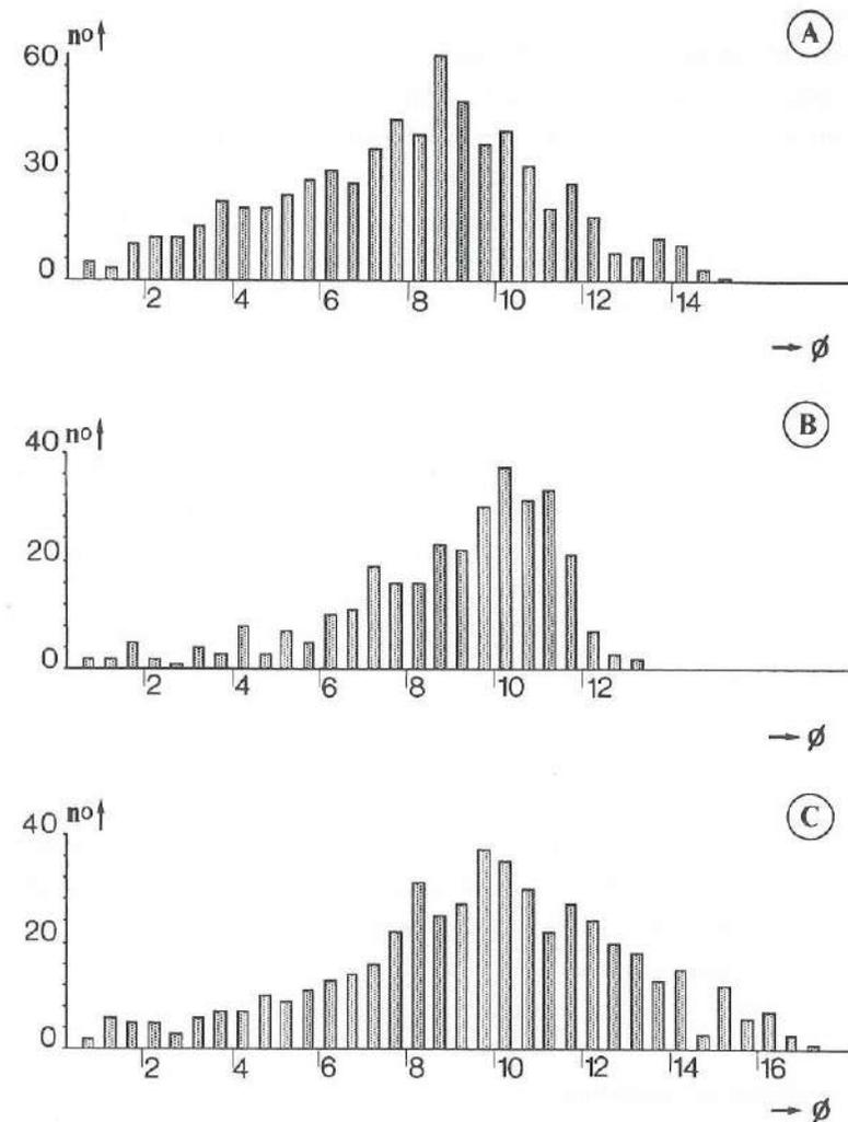
Fig. 1. Distribution of the pore diameters in the implants made of Estane<sup>R</sup> polyether urethane (a), polypropylene oxide (b), and HPOE/PBT segmented polyether polyester copolymer (c).
