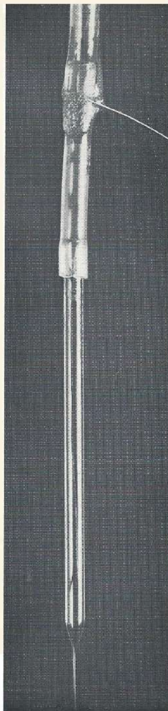
Fig. 3-2. The distal part of the measuring polythene cannula, the connective piece and the microcannula; note the silver wire entering the system between the polythene measuring cannula and the connective piece.
