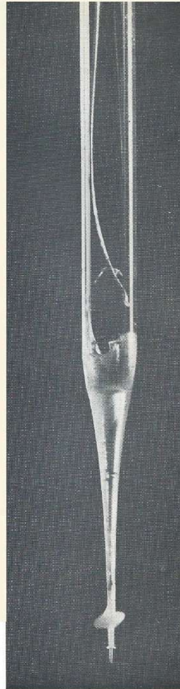
Fig. 3-7. The microcannula after retraction following a successful measurement. The upper and the lower ring of contact adhesive are the results of encounter with the round window and basilar membrane, respectively.
