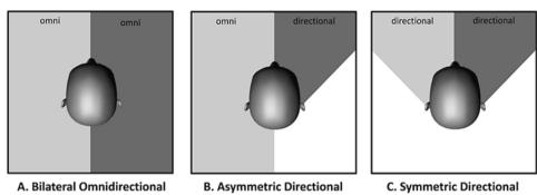
Schematic illustration of bilateral omnidirectional (A), asymmetric directional (B) and symmetric directional (C) configurations. Online available at: doi:10.1371/journal.pone.0160829.g001
