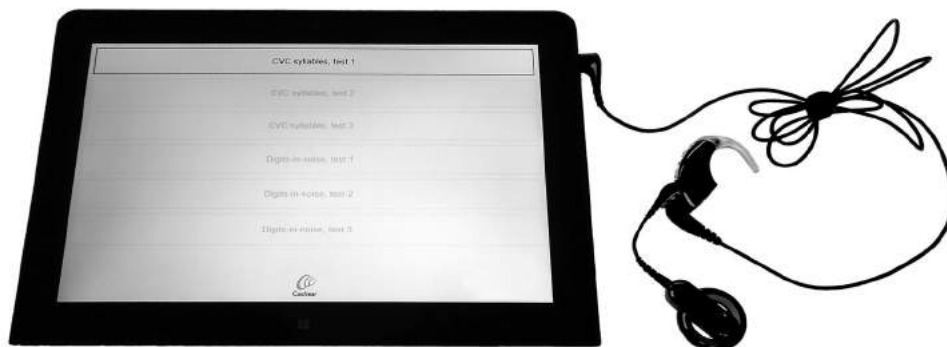
Figure 2. Experimental setup with a CI connected to a tablet computer using a PAC.
