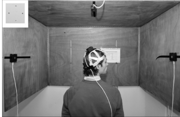
Figure 4.2: Experimental set-up for the head movement test. The cue display, positioned in front of the subject, is shown in the upper left inset. This display indicated the direction of the required head movement. Three target displays are visible; the fourth was positioned below and in front of the subject. The subject wore a movement registration device to measure head position and velocity.
