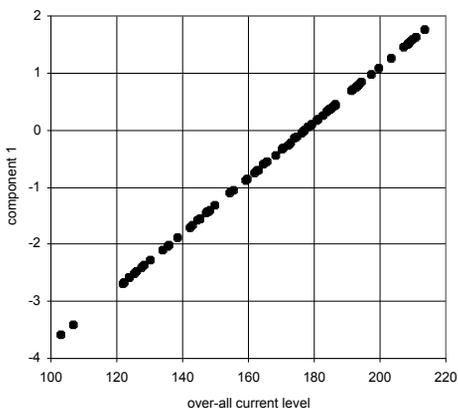
Figure 2: Relation between the scores for component 1 and the average level across all electrodes for all individual data contributing to Fig. 1 except those for T-min. An increase of the score for component 1 by one unit corresponds to about 20 current units.
