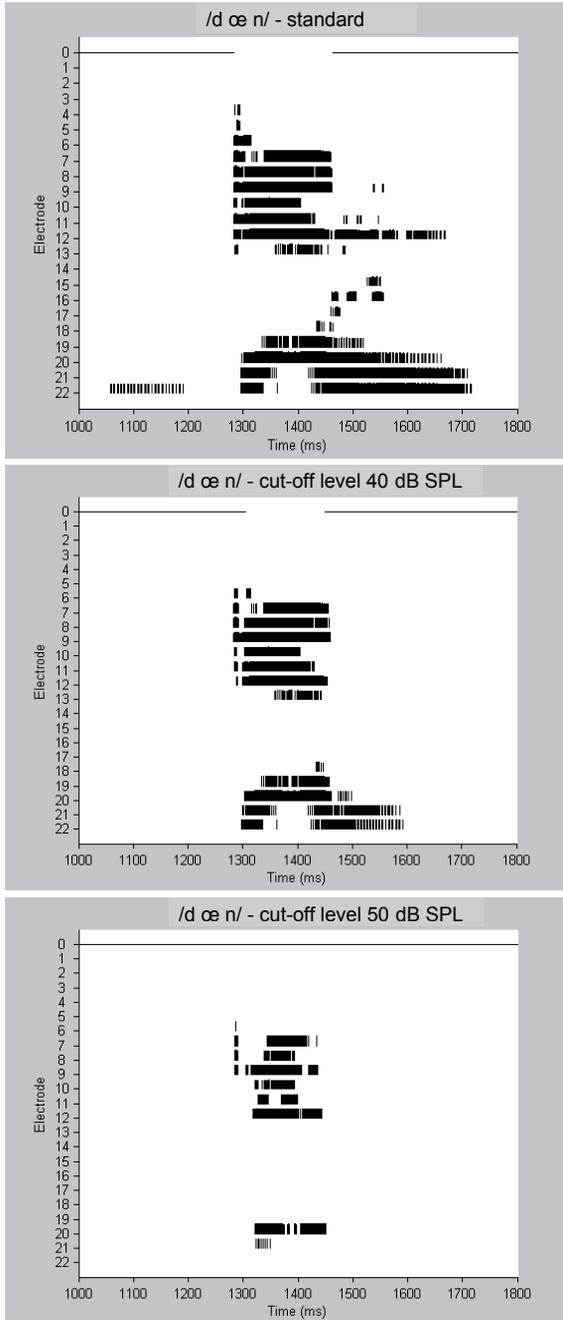
Figure 3: Electrodiagram (this is the stimulation pattern in time for each electrode) of the word /d œ n/ presented at 60 dB SPL using the simulation model with standard LGF and the LGF-manipulated strategy at cut-off levels of 40 and 50 dB SPL, corresponding to 58 respectively 80% of the EDR.
