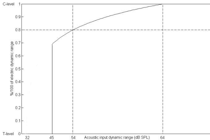
Figure 2: Acoustic-to-electric amplitude mapping according to the manipulated LGF. In this example a cut-off level of 45 dB SPL, corresponding to 69% of the EDR, is shown.
