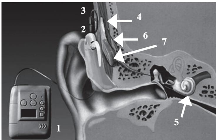
Figure 1: External and internal components of the cochlear implant (reprinted with permission from Cochlear Company). Externally are (1) the speech processor with (2) the microphone behind the ear and (3) the external coil. The implant consists of (4) an internal coil, (5) the electrode array placed in the cochlea, (6) the reference electrode MP1 placed beneath the temporal muscle, and (7) the reference electrode MP2 on the metal housing of the implant.
