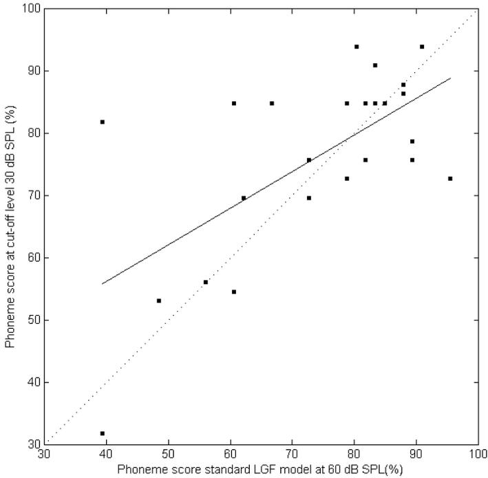
Figure 6: Relation between the individual phoneme score obtained with the standard LGF model at 60 dB SPL and with a cut-off level of 30 dB SPL. The solid line represents a linear least square fit. The dashed line represents a one-to-one linear relation.
