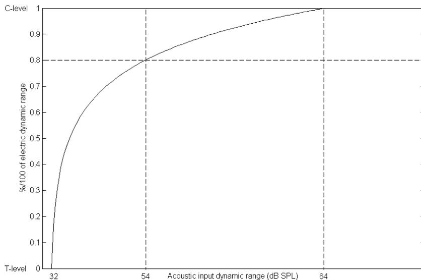
Figure 1: Acoustic-to-electric amplitude mapping according to the standard loudness growth function (LGF). The Q-parameter value determines the percentage of the EDR from C-levels downwards onto which the upper 10 dB of the acoustic speech range is mapped. In this example the Q value is at its default setting of 20. The base level determines the acoustic input dynamic range and thereby the lowest input level that results in a stimulus at T-level.
