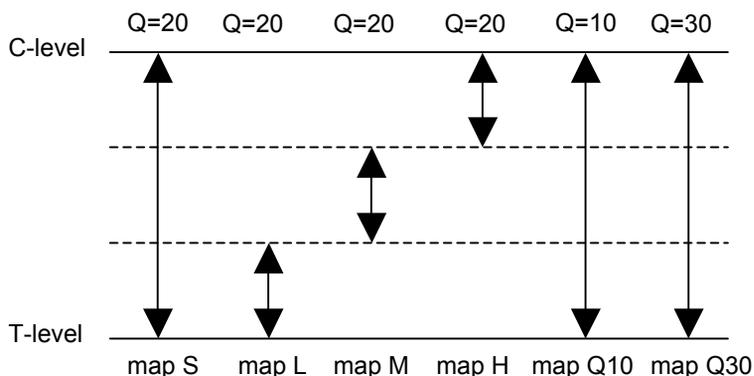
Figure 2: Standard map S and the five experimental maps L, M, H, Q10, and Q30. In map S, L, M, and H a Q value of 20 was used. In map L, the lower one-third of the EDR was used, in map M the middle, and in map H the upper third. In map Q10 and Q30 the full EDR was used, and the Q value was decreased to 10 in map Q10 and increased to 30 in map Q30.
