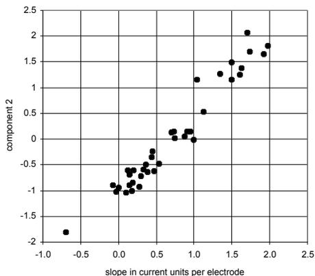
Figure 3: Relation between the scores for component 2 and the slope of the profiles across all electrodes for the individual T-, C- and ECAP profiles contributing to Fig. 1. An increase of the score for component 2 by one unit corresponds to a slope of about 2 current units over a 3-electrode distance.
