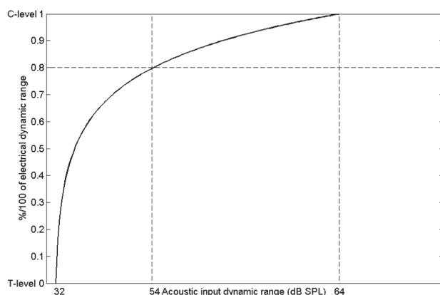
Figure 1: Acoustic-to-electric amplitude mapping according to the standard loudness growth function (LGF).
