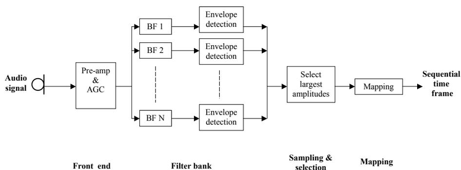
Figure 2: Block diagram illustrating the ACE strategy. Pre-amp is the pre-amplifier, AGC is the automatic gain control, BF are the bandpass filters.
