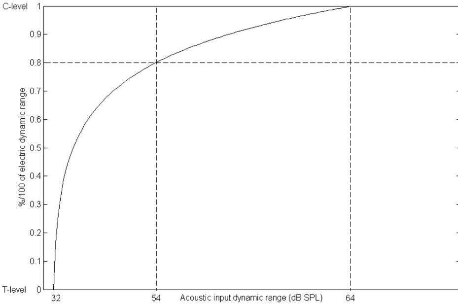
Figure 3: Acoustic-to-electric amplitude mapping: loudness growth function (LGF). This is the standard LGF setting, using a Q-parameter value of 20 and a base level of 4. The Q value of 20 implies that the upper 10 dB of the acoustic input range is mapped onto the upper 20 % of the electrical dynamic range. The base level of 4 results in an acoustic input dynamic range of about 32 dB SPL.
