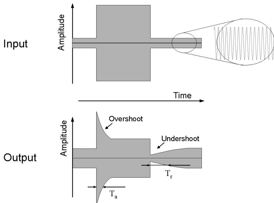
Figure 1.11: *Dynamic characteristics of compression. The upper panel shows the envelope of an input signal, in this example a sine wave which is modulated by a square wave. Compression in hearing aids typically reacts to level changes of the envelope of the input signal, and not to the fine structure (the sine wave). The lower panel shows the corresponding output signal.  $T_a$  = attack time;  $T_r$  = release time.*
