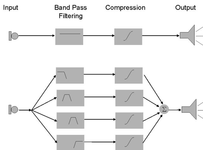
Figure 1.13: Schematics of compression. The top panel shows single-channel compression, the bottom panel shows multi-channel compression.
