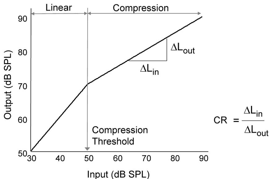
Figure 1.10: *Input-output curve of a compression system. Compression ratio (CR) is defined as the change in input level ( $\Delta L_{in}$ ) relative to the change in output level ( $\Delta L_{out}$ ).*
