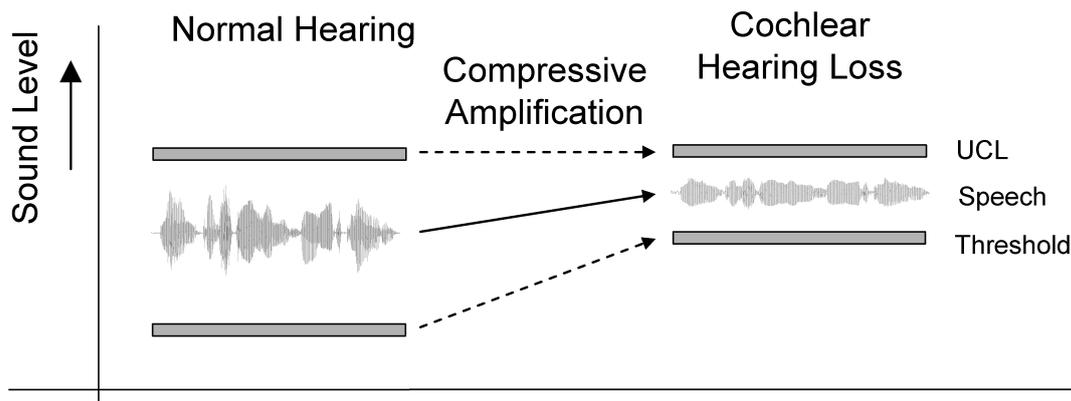
Figure 1.8: *Speech hardly fits into a small dynamic range. Compression of the speech signal can place speech within the residual dynamic range of the hearing-impaired listener.*
