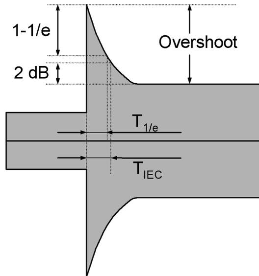
Figure 1.12: Different definitions of time constant.  $T_{IEC}$  represents time constant as defined by IEC 60188-2;  $T_{1/e}$  is our mathematical definition.
