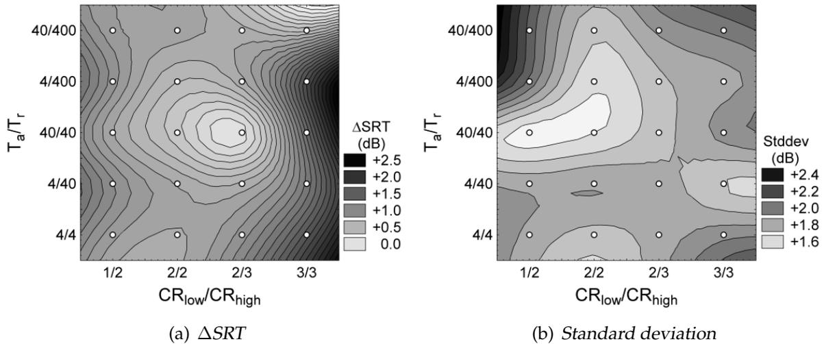
Figure 2.6: Contour plots for two-channel compression. Experimental data was available for every grid point (o). The intermediate values were calculated by a distance weighted least squares interpolation.
