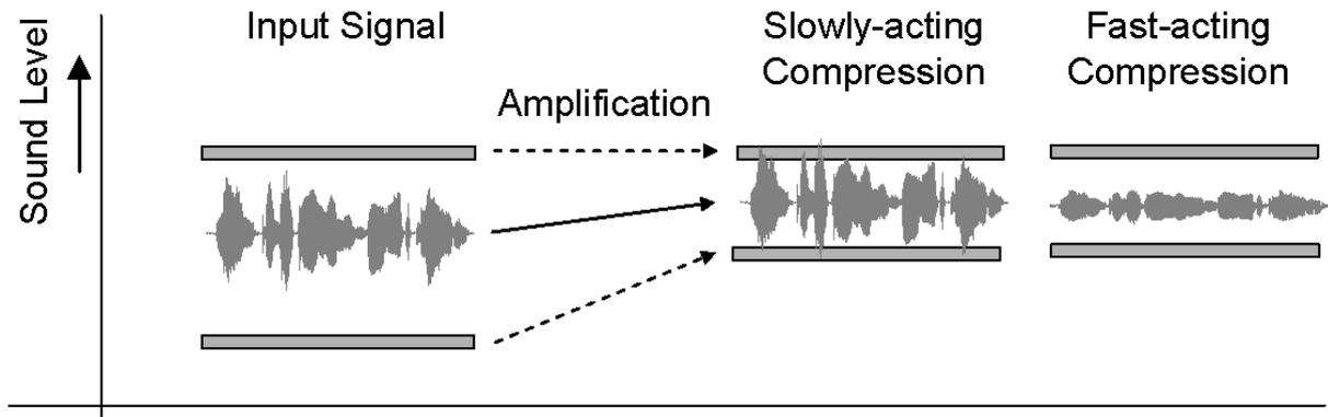
Figure 1.16: Both slowly-acting and fast-acting compression lift the speech above the elevated threshold. Fast-acting compression additionally reduces the dynamic range of speech itself.
