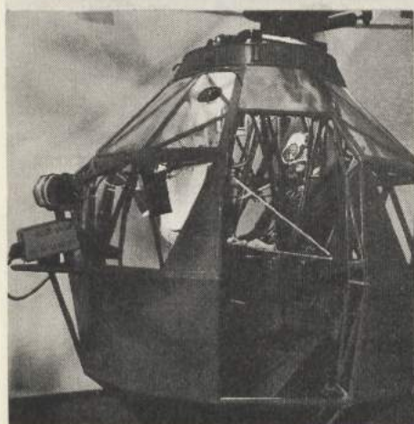
Fig. 1. APPARATUS. The staircase is hoisted out of the centrifuge pit when the centrifuge is used. In the gondola the subject is seen, wearing his mask and biting the dental impression, the fixing mechanism of which is not well visible. The subject holds the endless wire by which he can move the disc, which is shown separately. At the left (front) of the gondola is the TV camera viewing the other, white side of the disc; the calibration on this side of the disc is invisible in the reproduction.
