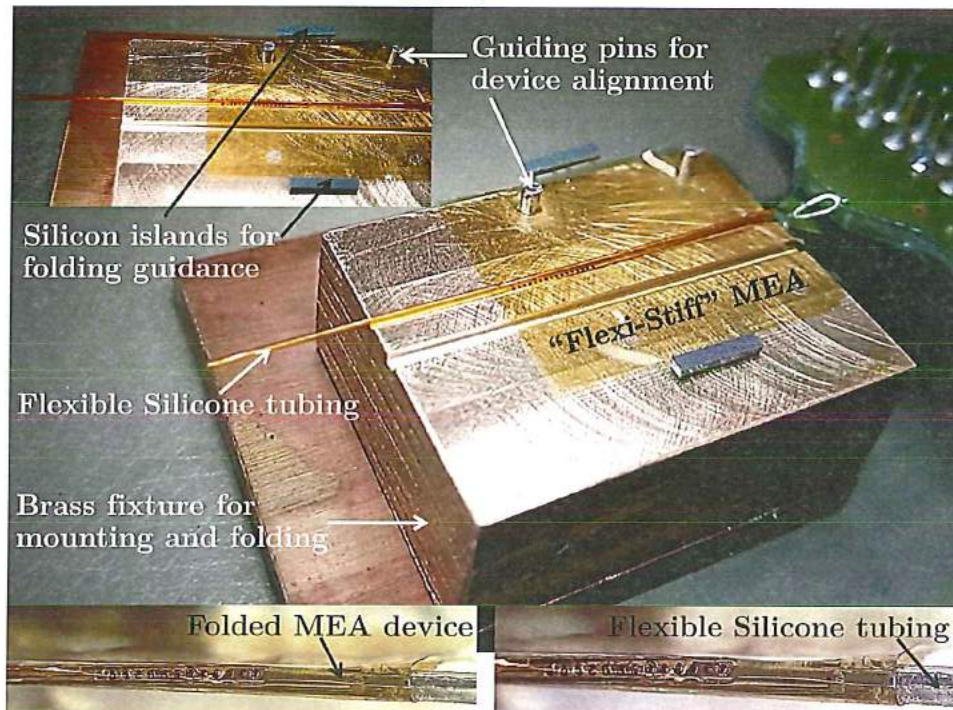
Figure 7.6 Mounting and folding of the "Flexi-Stiff" MEA.
