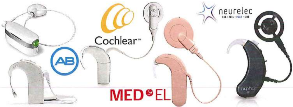
Figure 2.15 The present available range of CI speech processors from 4 manufacturers: from left to right: Advanced Bionics – Neptune and Naida CIQ70; Cochlear Corporation Ltd., – Nucleus® 5 Sound Processor; MED-EL – Sonnet Audio Processor; Neurelec (Oticon Medical in 2013) – Saphyr processor.
