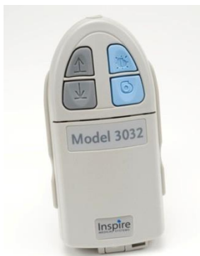
Figure 12: Patient sleep remote – used to turn the therapy on/off, as well as allow amplitude adjustments within a controlled range
