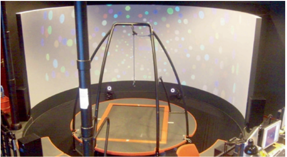
Fig 7.2 The CAREN motion platform (MOTEK, Amsterdam, The Netherlands) is a hexapod system, with a treadmill and four force plates underneath it. The 6 m semicircular screen enables a 180° field of view. There are twelve motion sensitive true infrared cameras (VICON) located around the platform and they respond to reflective markers.
