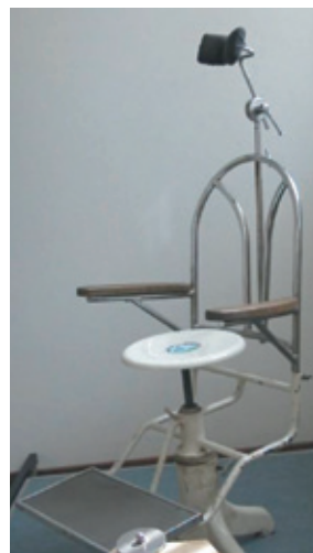
Fig. 2.1 The hand-driven Barany chair was part of the SD training as provided by the RNLAf in the last century at Kampweg 2, Soesterberg. In 1988 the Barany chair was saved from the garbage dump and given to TNO. The chair got motorized and was for years active in SD demonstrations and in the desensitization protocol. In this form the chair was used in the present experiment.
