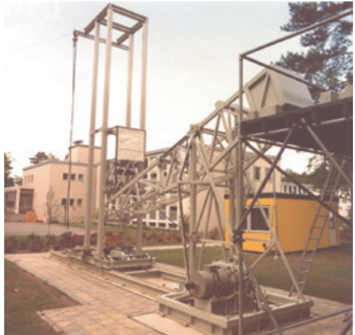
Fig. 7.1 The ‘Hotklots’, a motion simulator located at TNO Soesterberg from 1973-1975. By moving the tower the vertical motion could be damped from 4 m to 1.5 m. Maximum acceleration was 0.5 g. This device was originally built to simulate the dropping of concrete blocks from a cableway (to build a dam in the Oosterschelde). Investigated was the effect of the motion on the crew in terms of motion sickness. The political decision to keep the Oosterschelde open, implicated unfortunately the untimely end of this research project.
