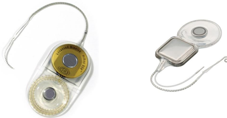
Figure 1. Examples of the internal parts: the receiver and electrodes
