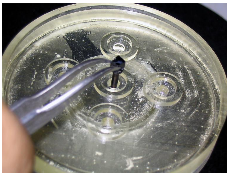
Figure 2: Demonstration of micro-manipulation task - holding a 2mm pin grasped between tweezers within a 4 mm hole, with both unsupported and supported wrists. The surgeons were asked to remain standing during this operation.
