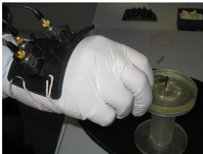
Figure 1: Placement of the 3 accelerometer's on the wrist.
