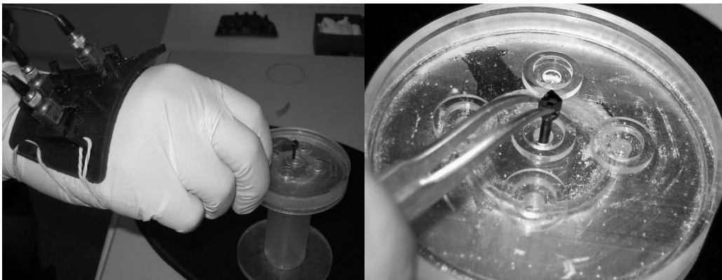
Figure 1: Accelerometer Placement and demonstration of micro-manipulation task of holding within a 4 mm hold a 2mm pin grasped between tweezers. The surgeons were asked to remain standing during this operation.
