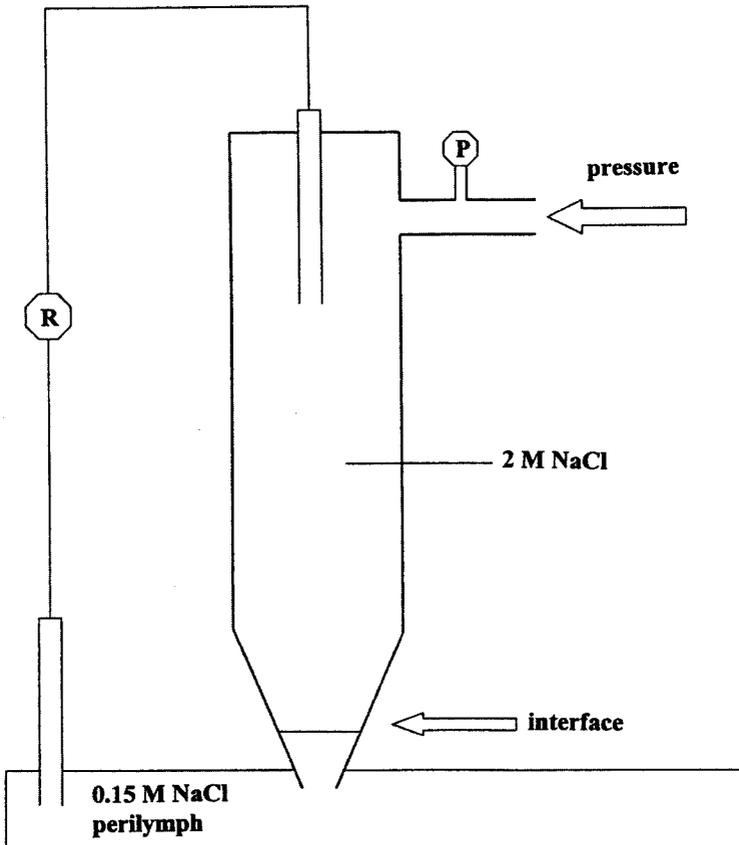
Figure 1 - Principle of the servo-controlled micropipette system
