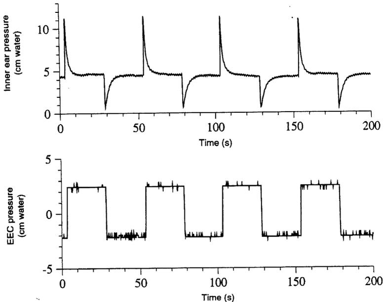
Figure 3 - Part of a measurement in which external ear canal pressure (lower panel) was manipulated with low frequency square wave pressure steps. Inner ear pressure in the perilymphatic compartment (upper panel) follows without a measurable delay; the system behaves as a high-pass filter.
