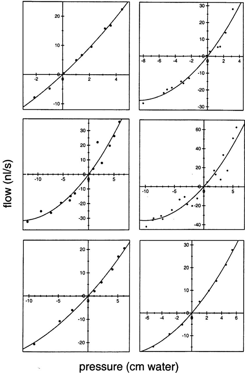
Figure 2 - Flow rates separately plotted against steady-state pressure increase or decrease  $\Delta p$  (in cm water) during infusion (see Figure 1) for all 6 guinea pigs. Solid lines: least-squares fits with second order curves to data points (black dots).
