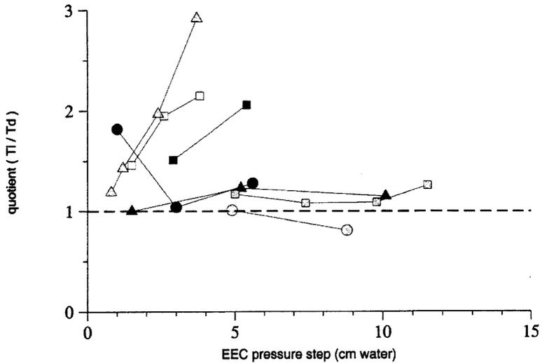
Figure 5 - Time constants for pressure increase ( $T_i$ ) divided by time constants for pressure decrease ( $T_d$ ), for different values of the amplitude of ear canal pressure change (connected symbols represent measurements in the same ear).
