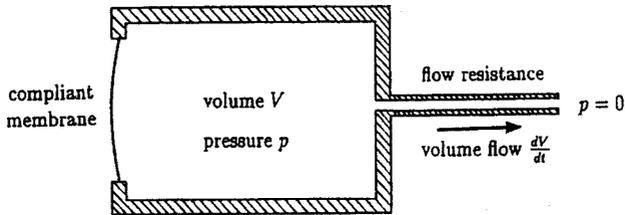
Figure 1 - Model for inner ear pressure release after volume increase. Immediately after volume increase inner ear fluid volume is  $V$  and pressure is  $p$ . This pressure returns to zero by fluid flow through the tube.
